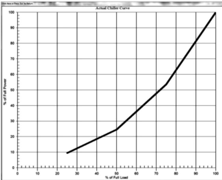
Figure 4. Actual Chiller Unloading Curve
