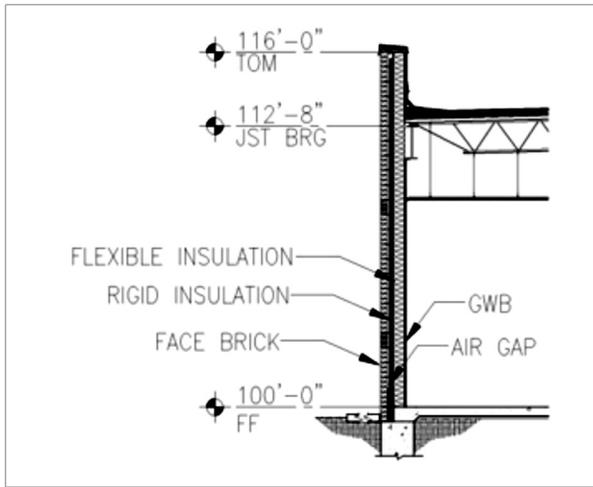
**Figure 1. Wall Section**
