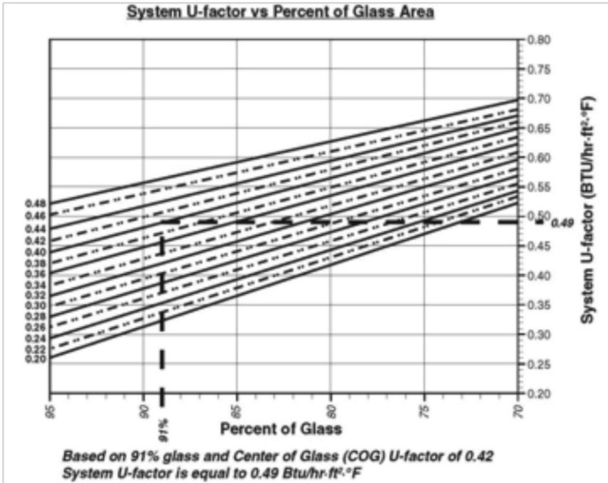
Figure 2. Glazing Assembly U-Factor
