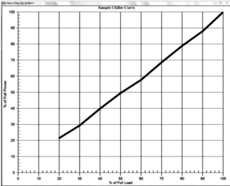
Figure 3. Sample Chiller Unloading Curve
