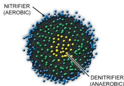
Figure 9 – Cross Section of Carbon Particle
